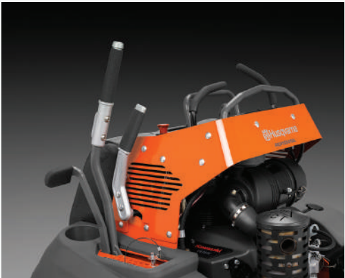
Dual Operator Presence Control (OPC) levers for more freedom of hand movement
